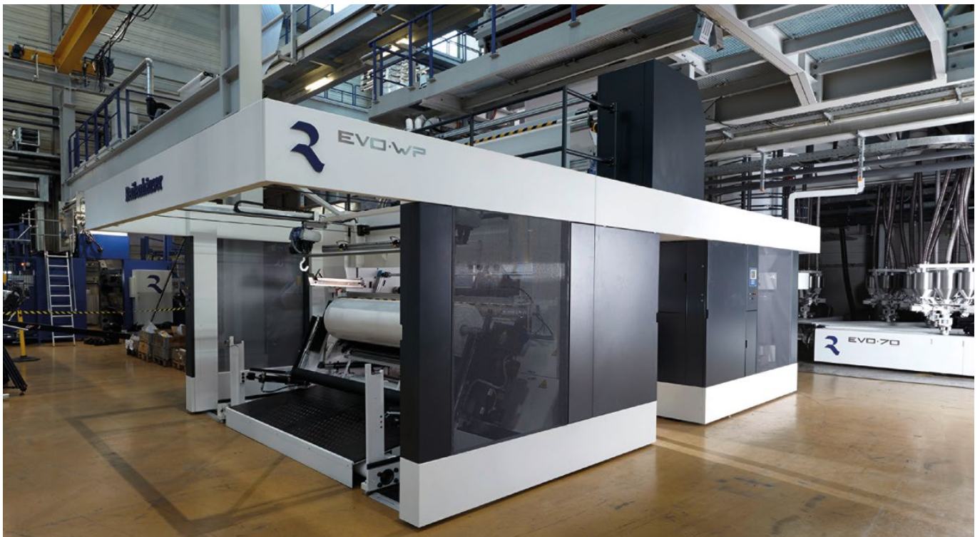
Modular design blown film winding system from the EVO-WP series with two winding stations.
